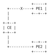
For example, CE is multihomed to PE1 and PE2. PE1 is elected as DF. All BUM flows are forwarded by PE1 when the link between PE1 and CE is operational. When the link between PE1 and CE fails, the BUM flows are discarded until PE2 is elected as DF.
