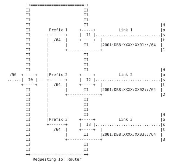
(In the above figure the Requesting IoT Router, with 4 links, is presented).
