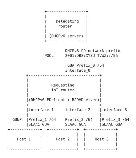
(In the above figure the scenario with 3 hosts connected to the Requesting IoT router is presented. Normally there are no number limitations of connected hosts.)
