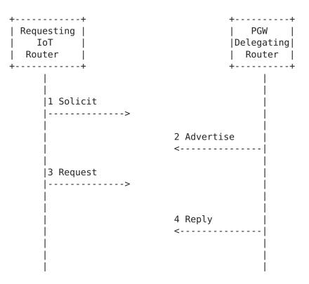
(In the above figure the full DHCPv6 message exchange mechanism between the ARM part of UE and PGW is presented.)
