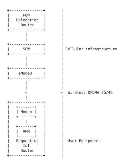
(The above figure descibes the model of the path followed by a DHCPv6 packet from IoT requesting router to the Delegating PGW router. The model is not a real infrastructure.)
