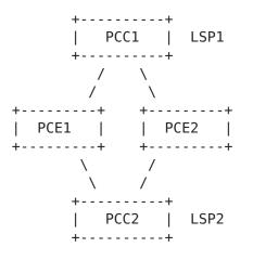
In the figure above, we consider a loadbalanced PCE architecture, so PCE1 is responsible to compute paths for PCC1 and PCE2 is responsible to compute paths for PCC2. When PCE1 triggers an LSP update for LSP1, it sends a PCUpd message to PCC1 for LSP1 containing the new parameters. PCC1 will take the parameters into account and will send a PCRpt message to PCE1 and PCE2 reflecting the changes. PCE2 will so be notified of the change only after receiving the PCRpt message from PCC1.
