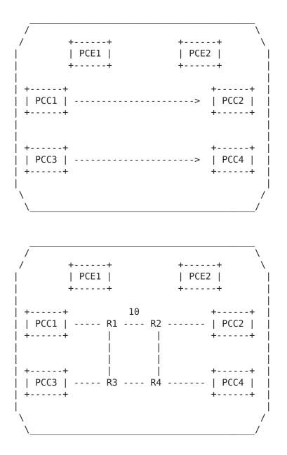
In the figure above, the requirement is to create two link-disjoint LSPs: PCC1->PCC2 and PCC3->PCC4. In the topology, all link metrics are equal to 1 except the link R1-R2 which has a metric of 10. The PCEs are responsible for the path computation and PCE1 is the active PCE for all PCCs in the nominal case.
