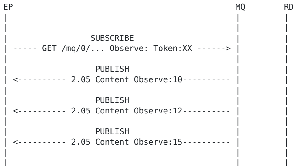
Figure 5: Client Role Endpoint SUBSCRIBE, Broker PUBLISH to Endpoint
