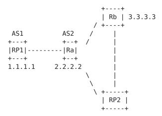
Where RP2 MSDP and MBGP peers with Ra (using 2.2.2.2) and with Rb (using 3.3.3.3). When the MSDP SA update arrives on RP2 from Ra, the MSDP RPF check for 1.1.1.1 passes because RP2 receives the SA update from MSDP peer 2.2.2.2 which is also the correct MBGP next hop for 1.1.1.1.
