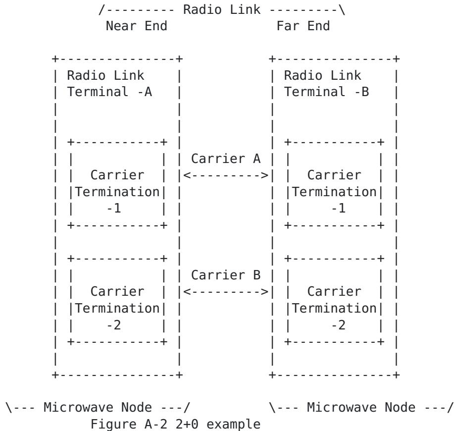
The following instance shows the 2+0 configuration of Near End node.
