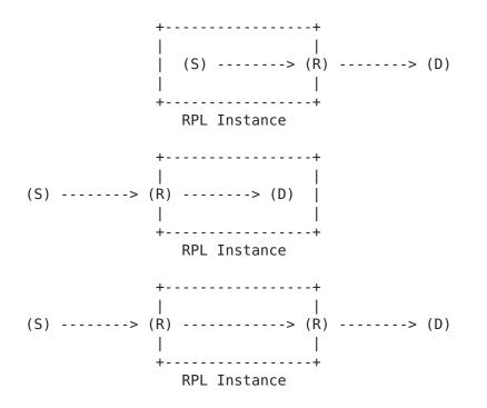
In the scenarios above, R may indicate a RPL Border Router (when connecting to other routing domains) or a RPL Router (when connecting
