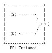
In the above scenario, datagrams travel from S to D through LBR. Between S and LBR, the datagrams are routed using the DAG built by RPL and do not contain a SRH. LBR encapsulates received datagrams unmodified using IPv6-in-IPv6 and the SRH is included in the outer IPv6 header.
