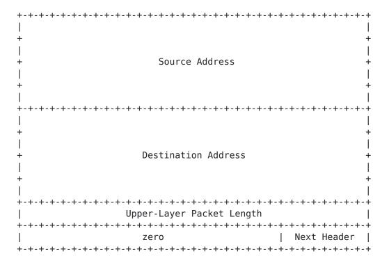
o If the IPv6 packet contains a Routing header, the Destination Address used in the pseudo-header is that of the final destination. At the originating node, that address will be in the last element of the Routing header; at the recipient(s), that address will be in the Destination Address field of the IPv6 header.
