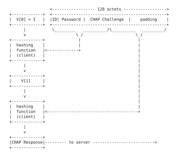
The following diagram illustrates the MD5 processing when using EAP-MD5-Tunneled. Note that the Client sends an intermediate result to the Tunnel Server, which completes the MD computation.
