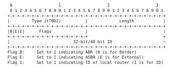
Undefined flags MUST be set to zero. The ID indicates the ID of a router. For a router not running IGP, the ID may be the 32-bit or 48-bit ID of the router configured.
