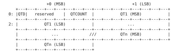
QTD: this bit indicates the direction of the packet. It MUST be clear (0) in a query and set (1) in a response.
