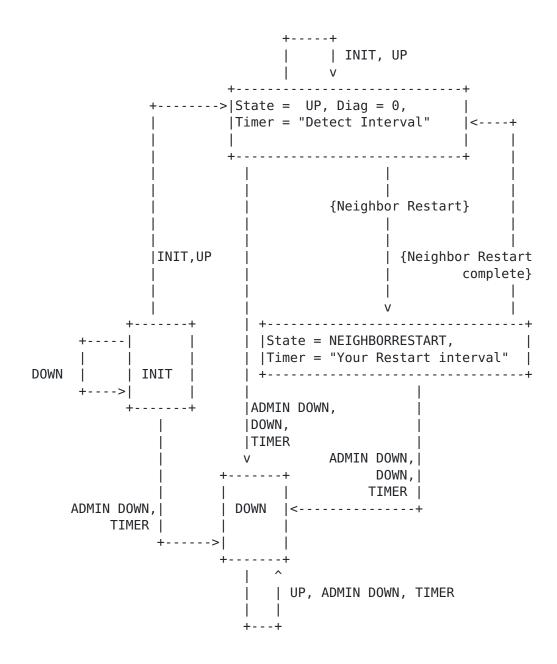
Note1: This state diagram holds only for BFD with GR extension as described in this document, which implies that "your Restart Interval" has a value greater than the Detection time value of the established session. This state machine must not be implemented.
