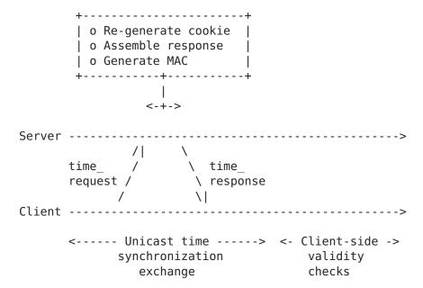
Procedure for unicast time synchronization exchange.
