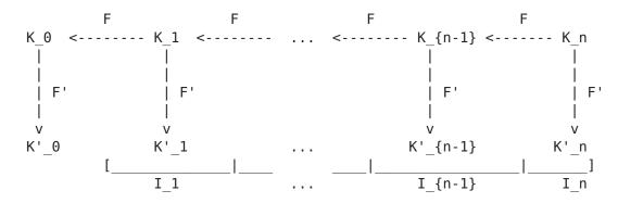
A schematic explanation of the TESLA protocol's one-way key chain
