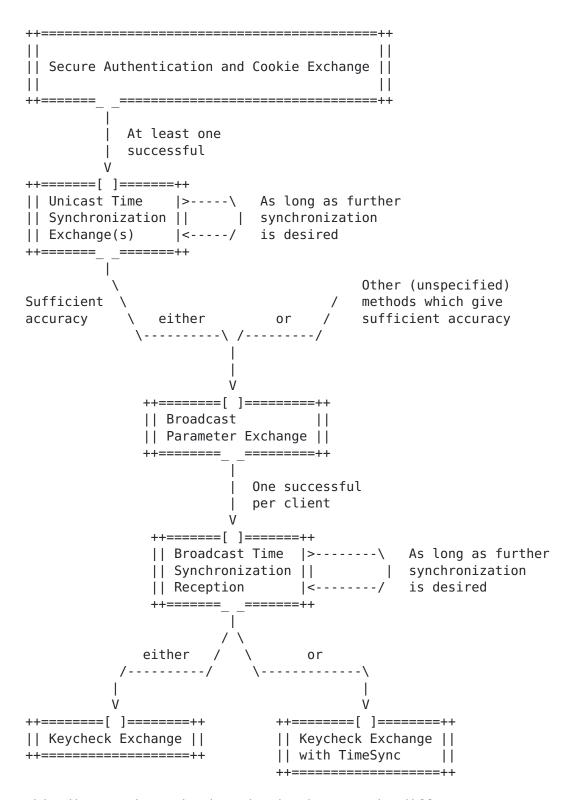
This diagram shows the dependencies between the different message exchanges and procedures which NTS offers.
