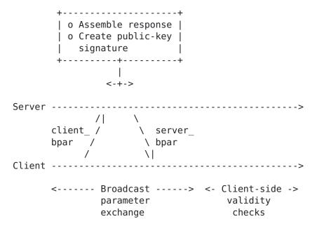
Procedure for unicast time synchronization exchange.
