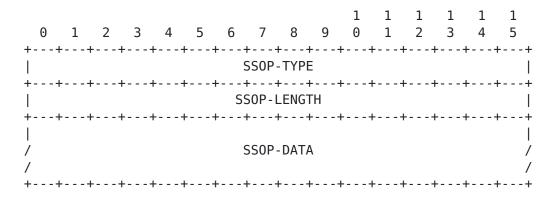
SSOP-TYPE: A 16 bit field in network order giving the type of the current Session Signaling TLV per the IANA DNS Session Signaling Type Codes Registry.
