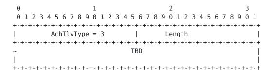
Figure 4: Label Switched Path Identifier
